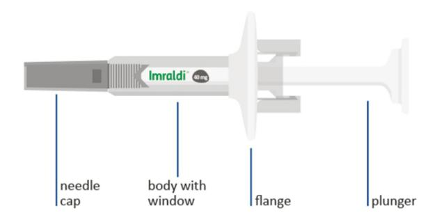
After you push the plunger all the way down, the needle will retract to help prevent needle stick injury.
