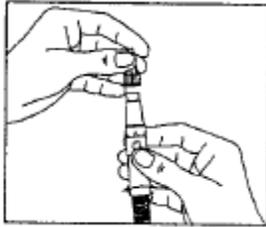
2. Attach the needle to the device by pushing the needle on to the tip of the device. Turn clockwise until it is firmly in place. The injection needle is enclosed in 2 protective caps. Pull off the outer protective cap of the needle.
