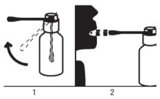
If after a number of applications the spray nozzle gets blocked the pump will malfunction. To correct this problem, remove the spray tube from the pump and clean it in a cup of hot water for a few minutes. Allow it to dry before fixing the tube back onto the pump.
