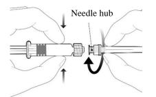
To attach the needle, connect the hub to the Luer Lock Adaptor and rotate a quarter turn clockwise until you feel it lock.
