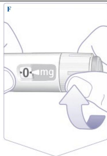
Make sure the flow check symbol lines up with the dose pointer.
