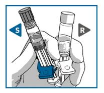
PULL the cap off the Solvent syringe.
