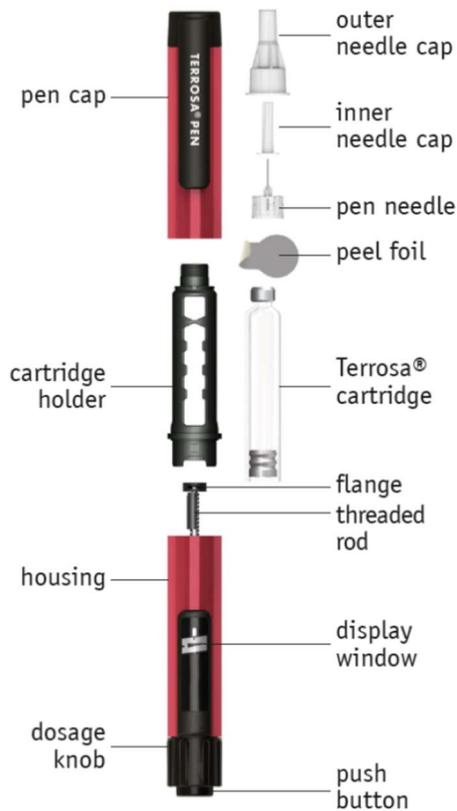
push button; display window; threaded rod; flange; Terrosa cartridge; peel foil; pen needle; inner needle cap; outer needle cap; pen cap; cartridge holder, dosage knob, housing
