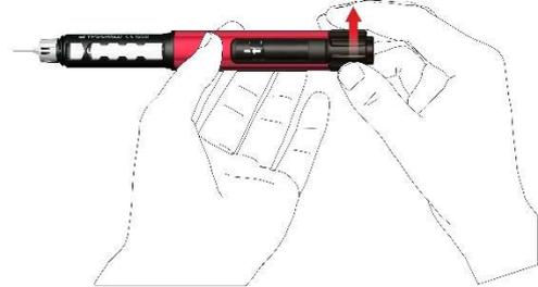
**Note:** If the cartridge contains less than 80 microliters, the dose knob cannot be turned clockwise up to the arrow sign. In this case, remove the pen needle, change the cartridge and proceed with priming according to the pen preparation steps.
