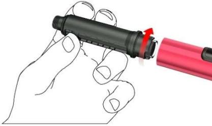
C: Remove the empty cartridge, in the case of changing cartridge. Insert a new Terrosa cartridge into the cartridge holder, with the metal crimped cap of the cartridge first.
