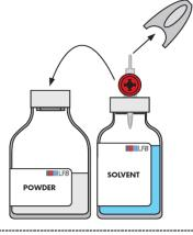
Remove the second grey protective sheath from the other end of the transfer system.
